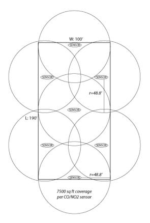
Note: All points inside the structure are within 50' of a Senva CO or NO2 sensor. This is a manufacturer recommendation. Consult local and state building codes to ensure coverage is adequate for the monitored space.
